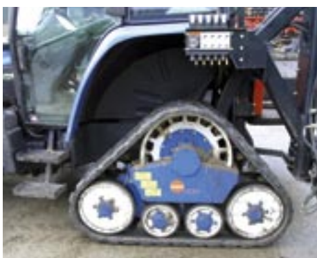
The rear wheels on Emerald Lawns' RoboMax harvester have been replaced by half-tracks which provide better flotation and more grip.
