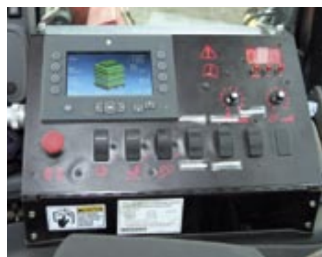
Driver's-eye view of the RoboMax's programmable control unit and stacking sequence display unit positioned to the right of the tractor seat.
